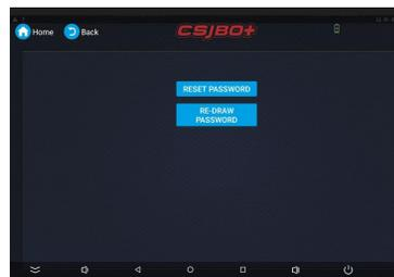
Click Reset verification password to enter the interface of reset verification password. The default password of the robot is csjbot. The administrator can verify the password according to the actual situation. The password length is between 8~16 digits. When the password are consistent in 2 times: the robot will remind that the password change is successful.
